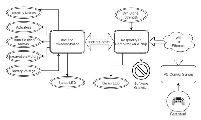
The figure above is a functional diagram for the subsystem of the robot. The project aims to develop the software of the subsystem and allow each component to communicate with the others. The hardware will be composed of three main parts, the Arduino, the Raspberry Pi, and the PC Control Station. The Arduino and Raspberry Pi will be on-board within the robot, and the PC Control Station will be separate and controlled by a human.
